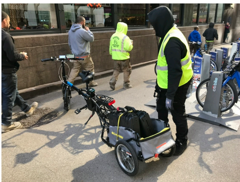
Figure 9: A staff undertaking battery swapping at a bikeshare station in New York City
