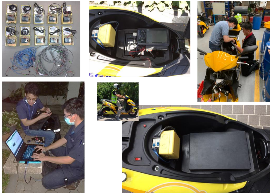
Figure 14: Design ECT (Energy Consumption Tracker) with demonstration pilot for e2w taxi in Thailand
